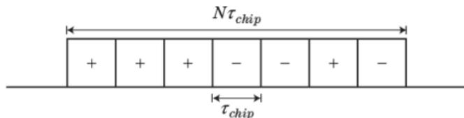
**FIGURE 20-23** ■ Biphas coded waveforms consist of chips exhibiting 2 possible phase states.
