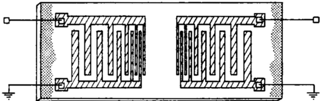
The device couples electromagnetic energy to acoustic waves, where the coupling is strongest when the distance between the metal fingers correspond to  $\lambda/2$  for the acoustic wave. Chirping is obtained by different acoustic propagation lengths. Works up to about 3 GHz, high insertion loss.
