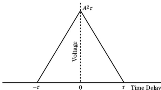
**FIGURE 20-2** ■ The simple pulse of duration  $\tau$  has a match filtered response of duration  $2\tau$ .
