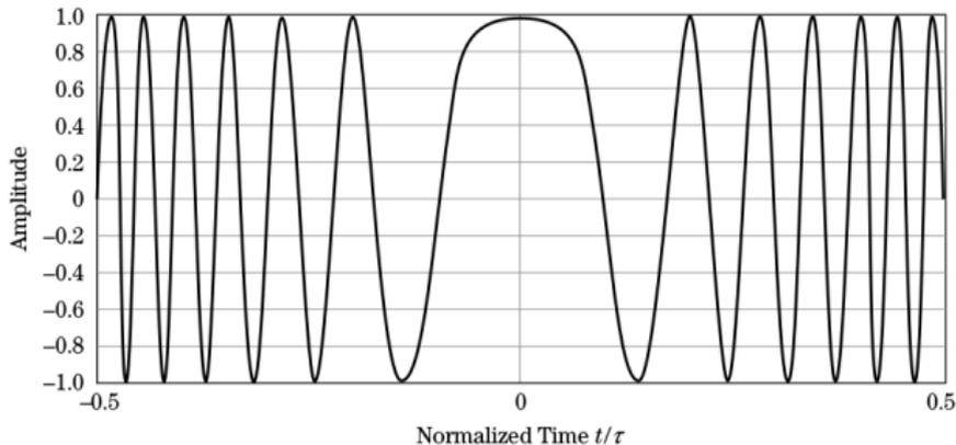
**FIGURE 20-7** ■ Time-domain response, within the pulse, of a linear frequency modulated (LFM) waveform with a time-bandwidth product equal to 50.
