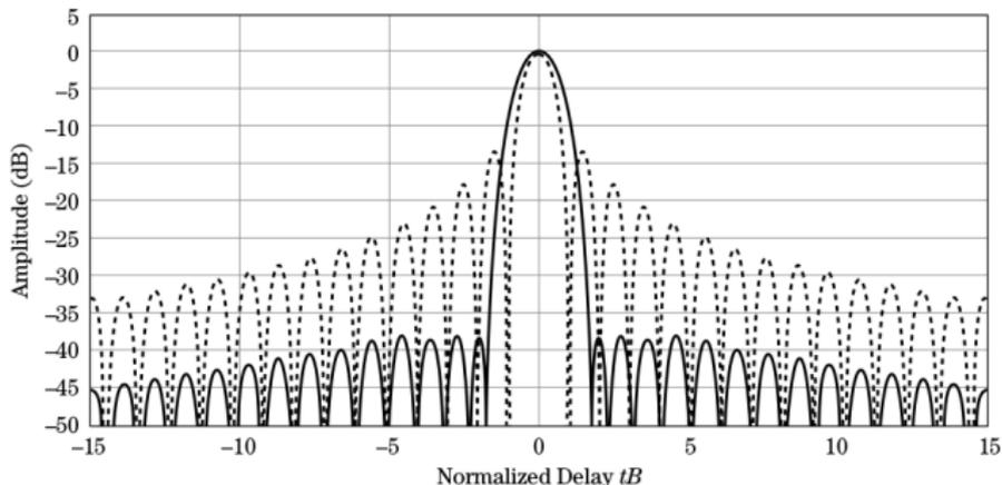
**FIGURE 20-13** ■ A  $-40$  dB,  $\bar{n} = 4$ , Taylor-weighted LFM waveform compressed response (solid curve) has significantly reduced sidelobes versus an unweighted LFM waveform response (dashed curve).
