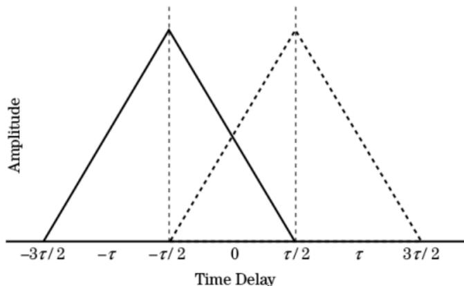
**FIGURE 20-4** ■ Individual responses from two point targets separated by the Rayleigh resolution.
