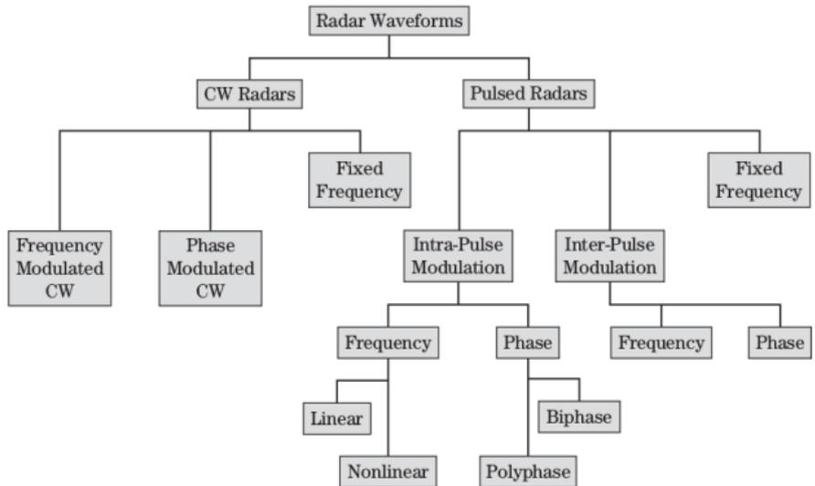
Many different waveforms are used in radars, taking many system requirements and constraints into account: bandwidth, power, Doppler tolerance, sidelobes, range resolution etc.
