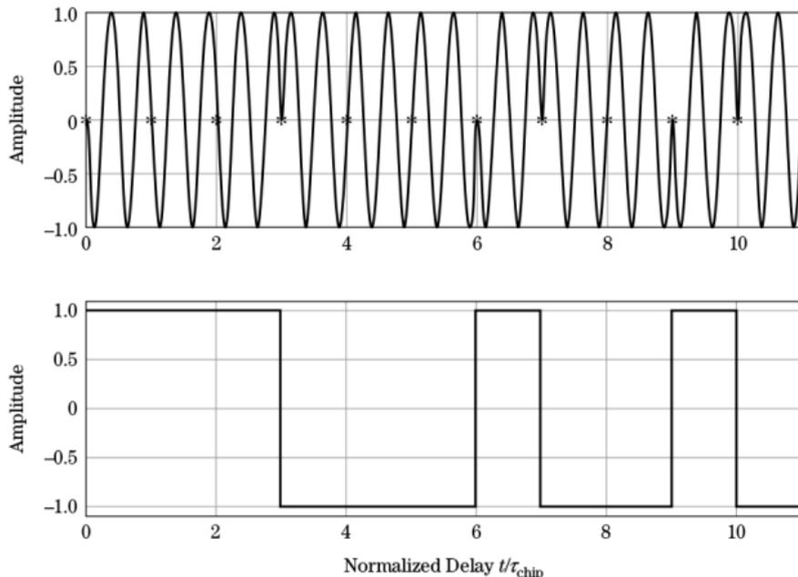
**FIGURE 20-25** ■ Baseband (bottom) and RF modulated (top) phase coded waveform of length  $N = 11$ .
