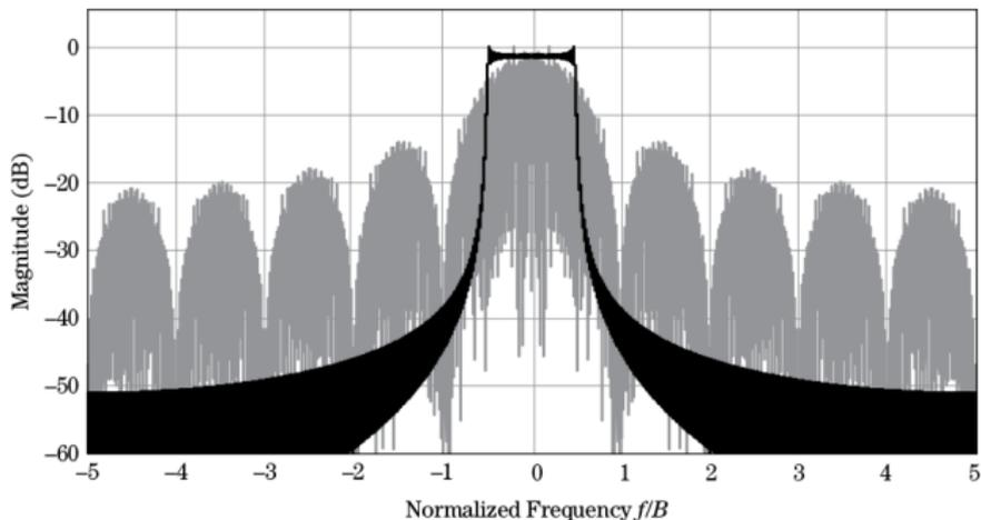
The wide spectrum of MLS can be attributed to the abrupt changes in phase. Can create an electromagnetic interference problem.
