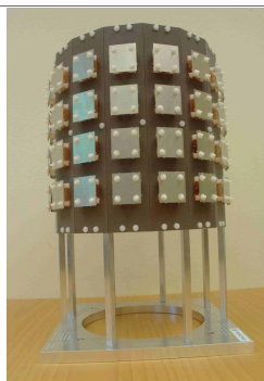
4x16 dual polarized circular patch array
