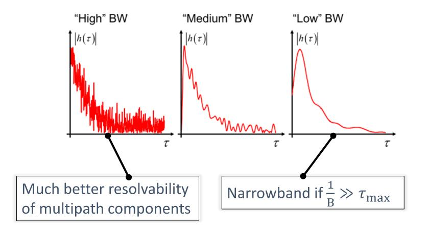
Power delay profile vs. frequency correlation function
