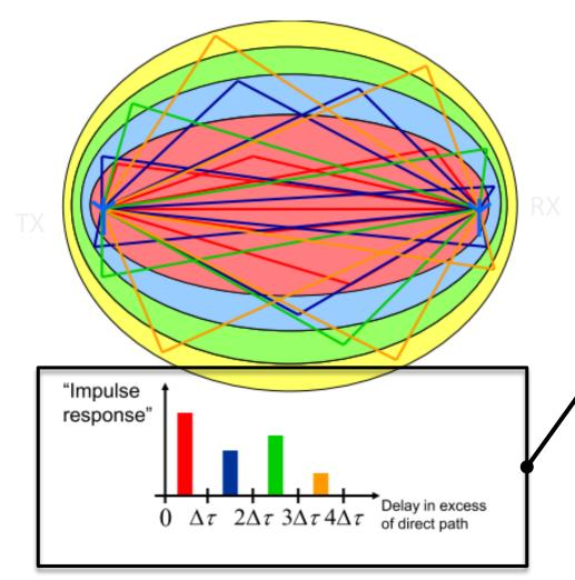
Discrete time-domain approximation to the impulse response of a wideband channel obtained by: dividing the impulse response into different time intervals (each containing multiple delays) and summing over the number of multipath components within each bin.
