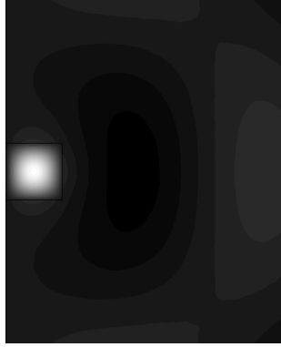
Figure 8.16: The magnetic field of the lowest resonant TM-mode. The frequency is f_r = 73.4 GHz for the cylindric resonator with \epsilon = 10 , radius a = 1 mm and height h = 1 mm.
