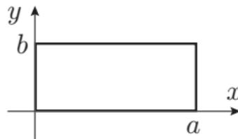
Rectangular waveguide  $a = 5 \text{ cm}$ ,  $b = 2\text{cm}$ .
