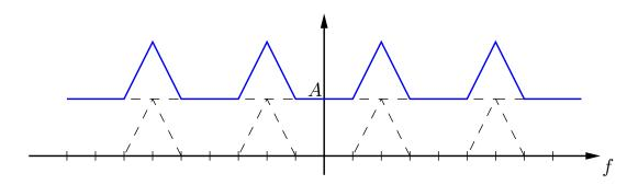
We can see that the shifted signals do not add up to a constant, which means that the ISI-free condition cannot be satisfied.
