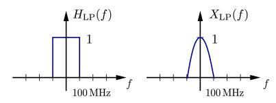
$W_{LP}$  should be between  $100\,\mathrm{MHz}$  and  $200\,\mathrm{MHz}$  to recover the baseband signal of user 2. Recall: we always use positive frequencies to measure bandwidth.
