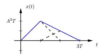
(c) We need to identify the largest  $R_s$  for which the shifted signals add to a constant. We obtain  $R_s = 5000$  symbols per second, and A has to be chosen as  $x_0/R_s$ .
