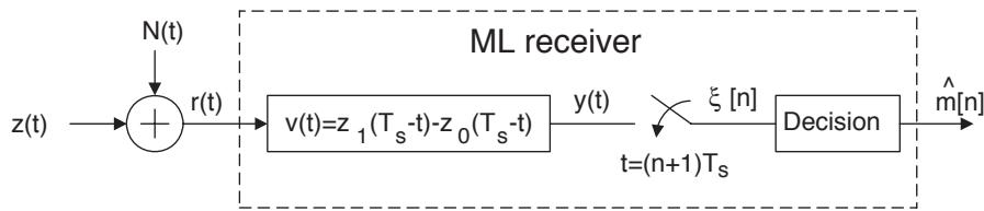
The ML receiver above is identical with Figure 4.10 on page 247 in the compendium. *The average received signal energy per information bit  $\mathcal{E}_b$*  is the same in the three figures, but *the noise parameter  $N_0$*  is different.
