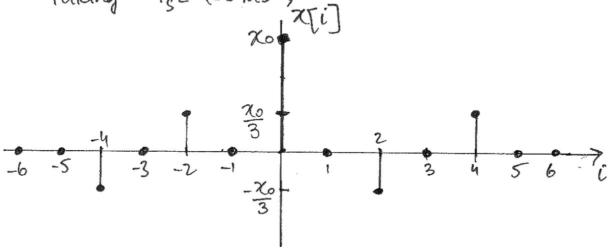
From the impulse response, it can be seen that for  $T_s = 300 \mu s$ , there will be no interference
