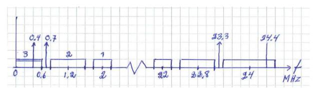
iii) Correct user signal (user 3) at base band in y(t). A disturbance at 400 kHz. Low pass filter bandwidth should be 600 kHz.
