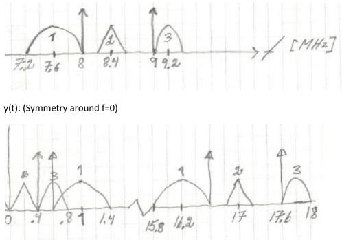
The choice of 8.6 MHz in the receiver is a bad choice. It should be 7.6, 8.4 or 9.2 (MHz), then the corresponding user signal will be found around the frequency f=0.
