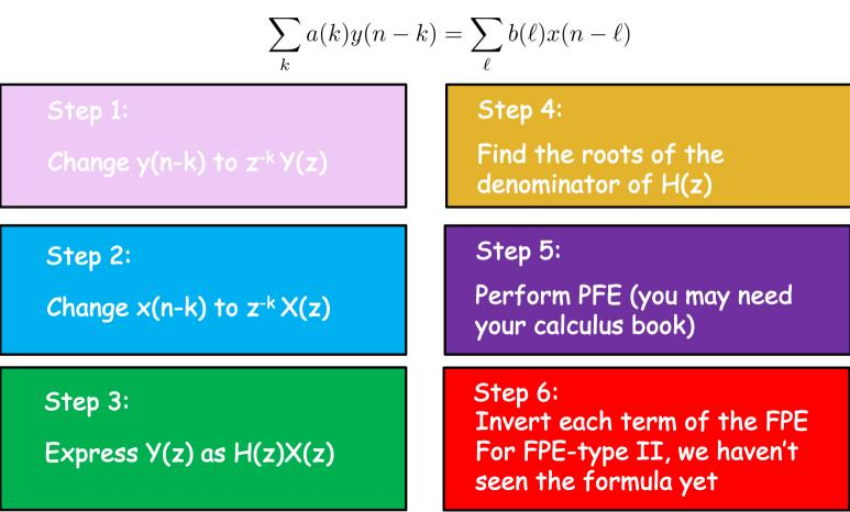
One further example: y(n) - 1.27y(n-1) + 0.81y(n-2) = x(n-1) - x(n-2)All signals causal
