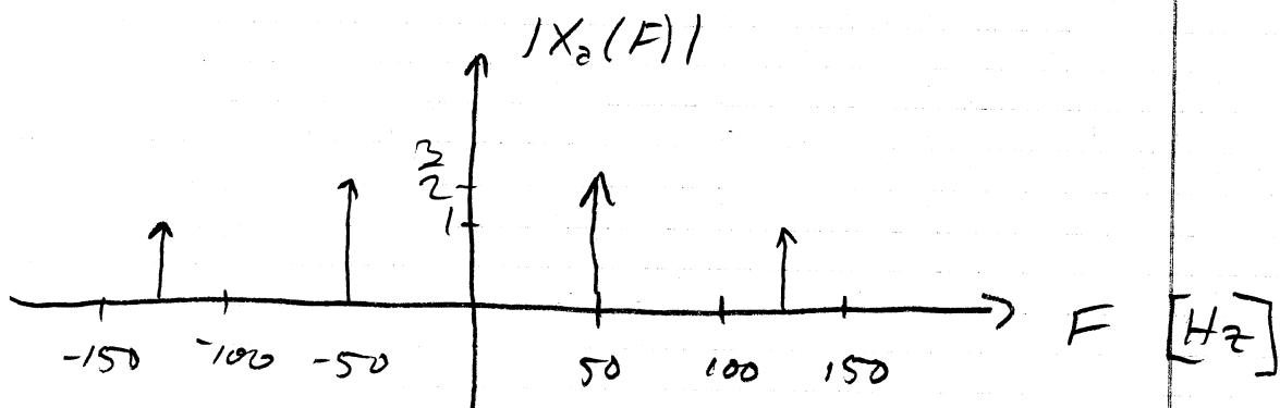
The plot of  $X(F/F_1)$  ( $F_1 = 200 \text{ Hz}$ )
