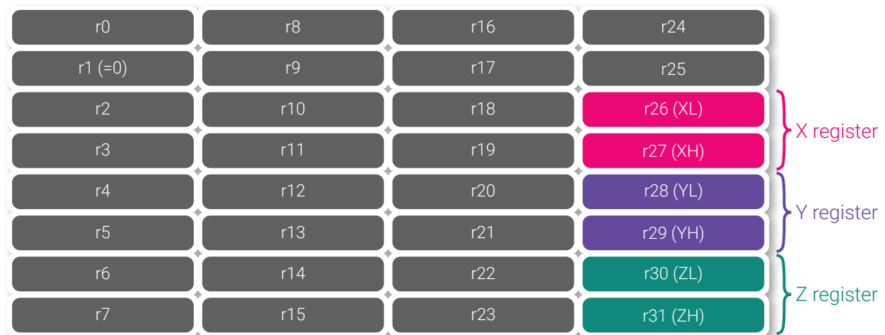
Figure 1: The register file in the processor with the X, Y and Z register highlighted.
