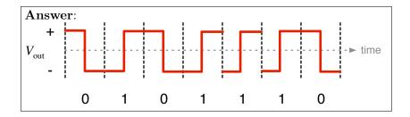
6.2 Following the convention established in Problem 5. The first symbol is to illustrate the state of the signal.
