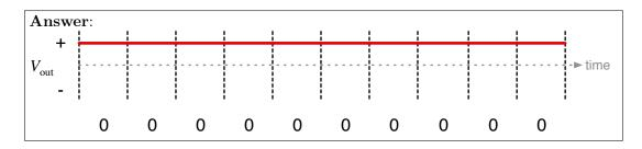
3.2 In a Manchester modulated signal, each bit i demarked by an output transition during the allocated bit duration (symbol) as opposed to a constant level seen in NRZ modulation. In the figure below a zero is represented by a falling edge, while a one is represented by a rising edge.
