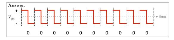
3.3 As you will see in Problem 5, Differential Manchester coding deals with transitions between symbols rather than output levels within a symbol. A sequence with all zeros is represented by the absence of symbol transitions, and the waveform is therefore identical to the Machester coded one in problem 3b.
