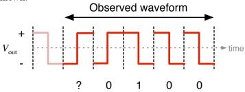
As you can see in the figure above, we do not know if first symbol is zero that transitions into a one, or the tail of a sequence of transitions representing several ones. Differential Manchester is used because a transition is less likely to be misinterpreted than a individual symbols by the receiver, given a noisy channel. Differential Manchester encoding is predominantly used in magnetic and optical storage.
