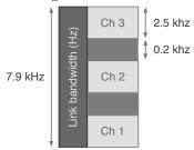
Subtracting the sum of the two guard intervals of 0.2 kHz each from the total allocated link bandwidth leaves us with the remaining bandwidth for the sum of the three channels, 7.9 kHz -  $2 \times 0.2$  kHz = 7.5 kHz. Furthermore, as there are three channels, each channel can be allowed a bandwidth of  $\frac{7.5}{3}$  kHz = 2.5 kHz.
