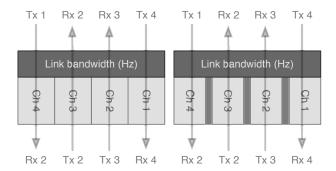
In this instance, it is specified that each channel needs a bandwidth of 4000 Hz = 4 KHz with a guard interval of 200 Hz = 0.2 kHz. Since there are five channels, we need four guard intervals to separate them. Moreover, this leaves us with a total link bandwidth of  $5 \times 4$  kHz +  $4 \times 0.2$  kHz = 20.8 kHz. See the figure below.
