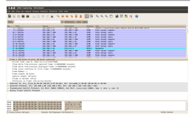
Captured frames are shown in real time in the main WireShark window. You find all captured frames in the upper window, one frame on each row. The frame capturing will continue until you stop it manually by hitting the Stop capture button in the upper left corner.
