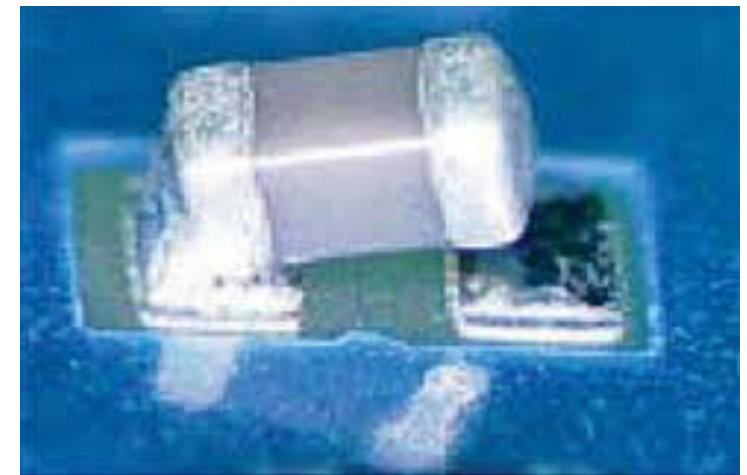
Fig. 1. With "tombstoning" only one side of a two-leaded chip component may be soldered to the target pad, but its other termination may not come in contact with the associated target pad. Photo courtesy of IPC-610
