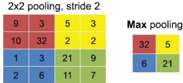
Fig. 3. Showing a Simplified Version of Max Pool Layer [1]
