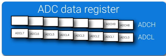
Figure 5.3: The ADC value is stored in the result registers.
