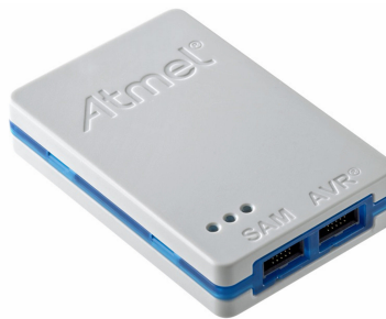
Figure 1.5: The Atmel-ICE programmer and debugger.
