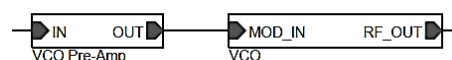
Figure 1 – Block view of the frequency modulator. Input is from the left and output to the right.
