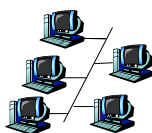
bus: coaxial cable
