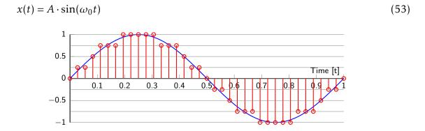
A resolution of *b* binary bits yields a total of  $2^b$  signal levels. If the maximum amplitude is *A* then the dynamic range becomes 2A.
