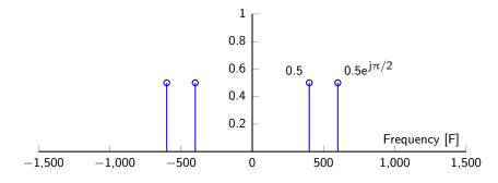
Spectrum after sampling (the discrete signal):
