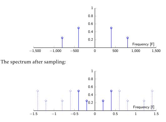
Folding distortion yields a "false" frequency at  $f = \pm 0.2$  corresponding to  $F = \pm 200$  Hz. For discrete signals in general, a frequency at  $f_i$  also appears at  $f_i \pm 1$ ,  $f_i \pm 2$ , and so on.
