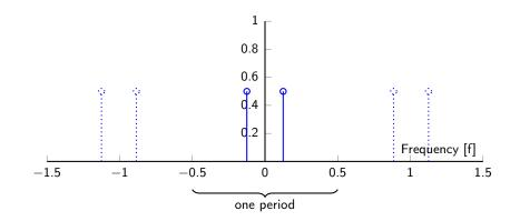
An example of frequencies and the periodic spectrum. The sampled frequency f' in the table is always  $-0.5 \le f' < 0.5$ .
