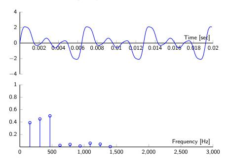
Clarinet with fundamental frequency  $F_0 = 156$  Hz and 13 harmonics.
