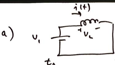
$$\text{Spule, si } V_L = L \cdot \frac{di}{dt} = v_i$$
