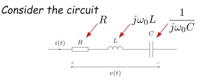
The current i(t) is a sinusoid of frequency  $f_0$  Hz. What is v(t)? Total (serial) impedance at frequency  $f_0 = \frac{\omega_0}{2\pi}$ :  $Z(\omega_0) = R + j\omega_0 L + \frac{1}{j\omega_0 C}$ Ohm's law gives:  $v(t) = Z(\omega_0)i(t) = (R + j\omega_0 L + \frac{1}{j\omega_0 C})e^{j\omega_0 t}$
