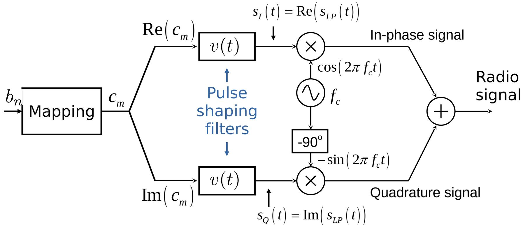
(Both the rectangular and the (root-) raised-cosine pulses are real valued.)
