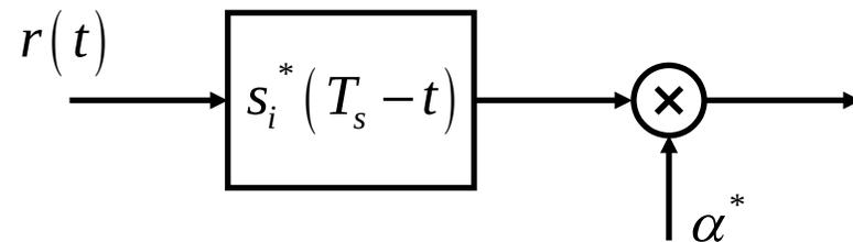
The real part of the output from either of these is sampled at  $t = T_s$
