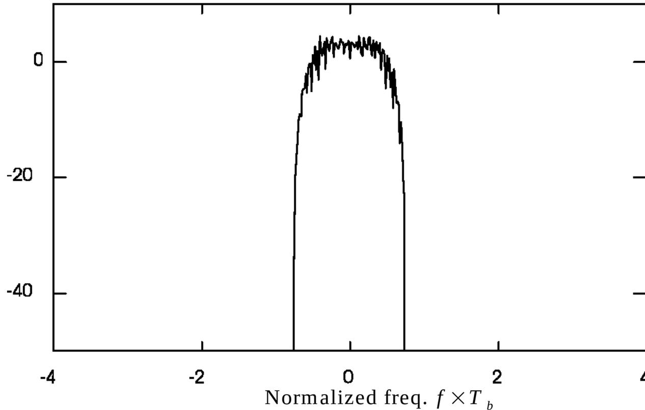
Much higher spectral efficiency than BPSK (with rectangular pulses).
