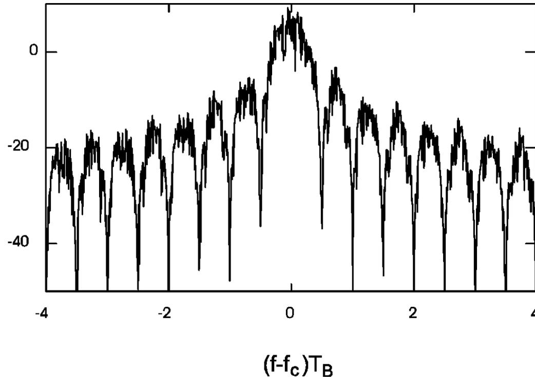
Twice the spectrum efficiency of BPSK (with rect. pulses). TWO bits/pulse instead of one.
