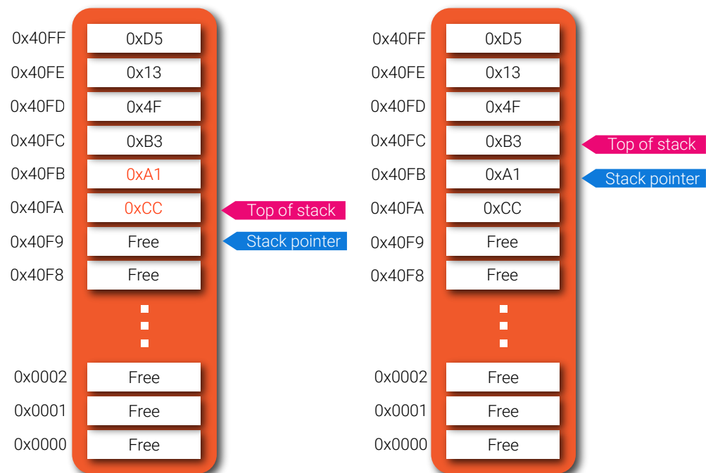
Figure 2.3: The stack before and after (right) the allocated bytes have been “returned”.
