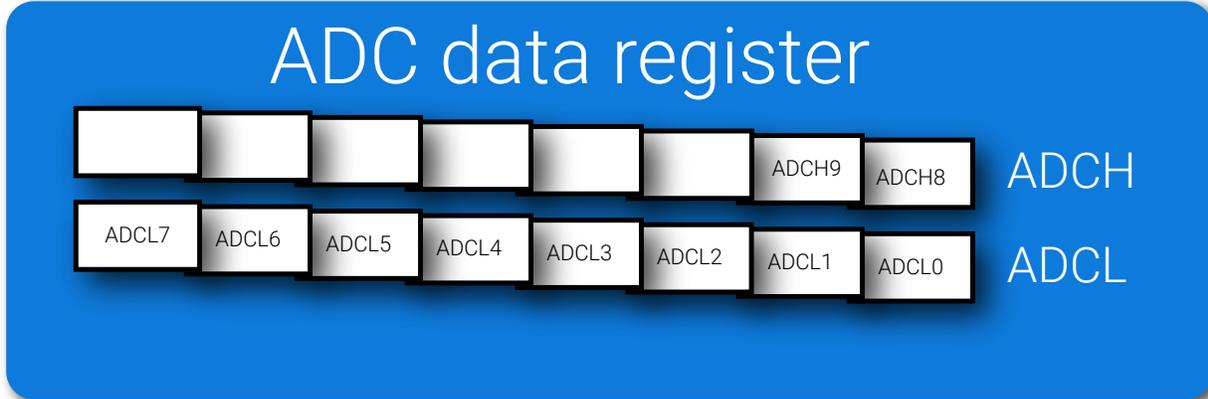
**Figure 4.3:** The ADC value is stored in the result registers.
