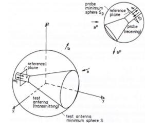
Experimental setup geometry
