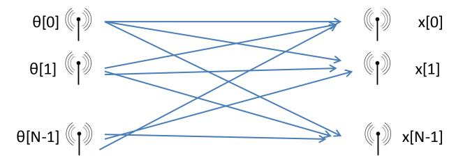
All channels are assumed Different due to the nature of radio propagation
