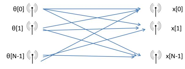
All channels are assumed Different due to the nature of radio propagation
