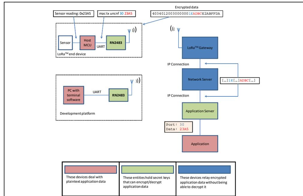
The flow of data can be followed as it gets generated by an end device and transported on the network.
