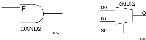
Figure 21: AND & MUX Symbols in XC4000X IOB
