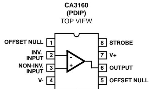
NOTE: CA3160 Series devices have an on-chip frequency compensation network. Supplementary phase compensation or frequency roll-off (if desired) can be connected externally between Terminals 1 and 8.
