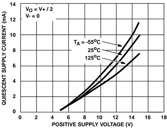
FIGURE 19. QUIESCENT SUPPLY CURRENT vs SUPPLY VOLTAGE
