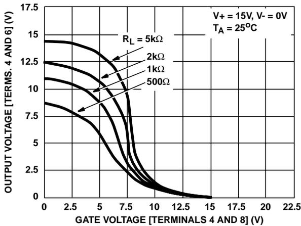
FIGURE 17. VOLTAGE TRANSFER CHARACTERISTICS OF CMOS OUTPUT STAGE
