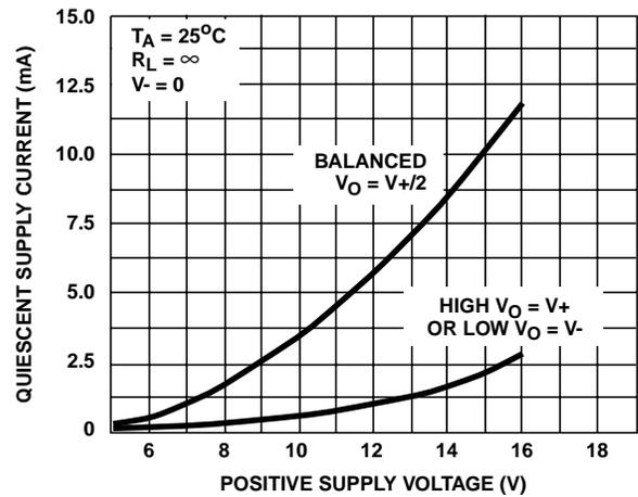
FIGURE 18. QUIESCENT SUPPLY CURRENT vs SUPPLY VOLTAGE
