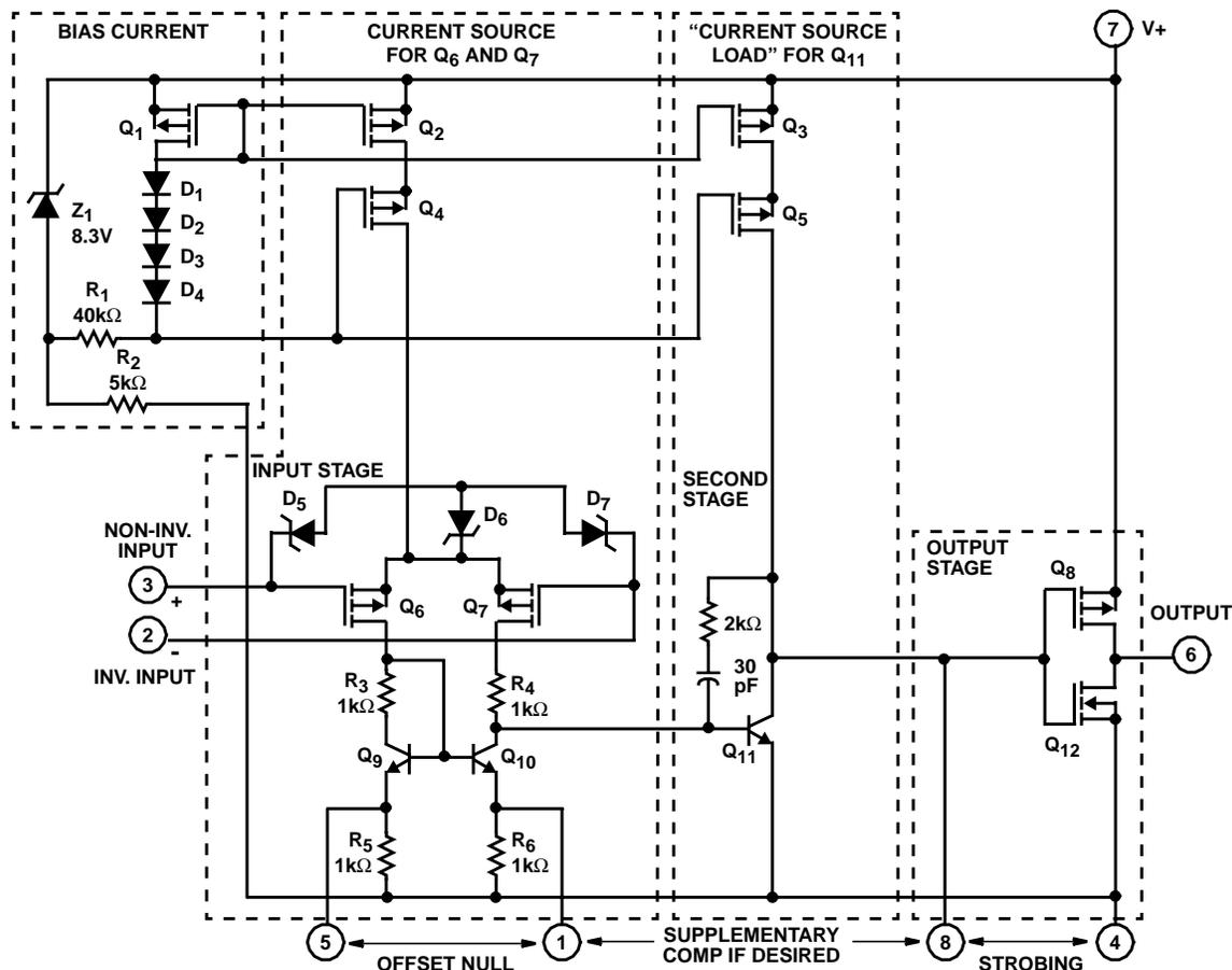
NOTE: Diodes D<sub>5</sub> Through D<sub>7</sub> Provide Gate Oxide Protection For MOSFET Input Stage.
