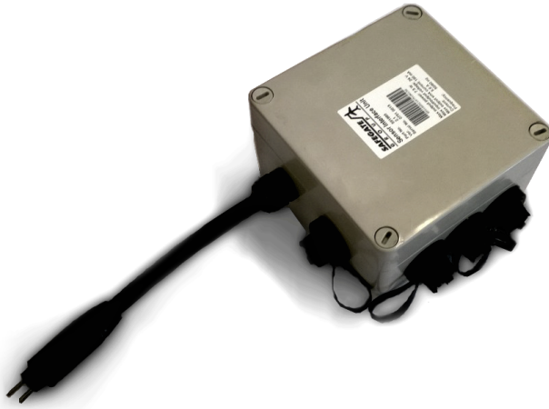
Figure 2.4: A sensor interface unit. The long cable is the connector to the isolation transformer and the four connectors are sensor ports.
