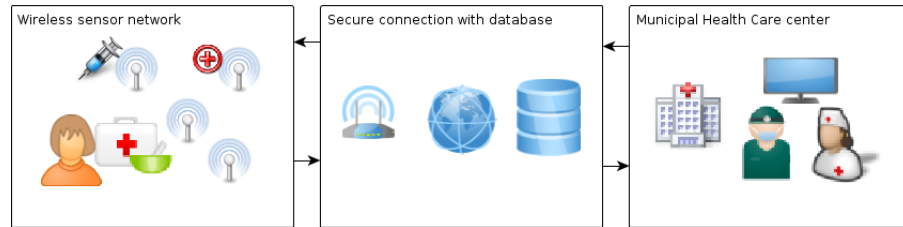
Figure 5.6: A ZigBee based system with an ISO/IEEE 11073 PHD Implementation
