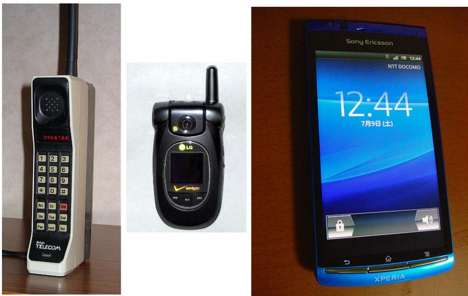
Figure 1. (Left) Motorola DynaTAC with whip antenna [1] (Middle) LG VX8300 with stubby antenna [2] (Right) Sony Ericsson Xperia with internal microstrip antenna [3]
