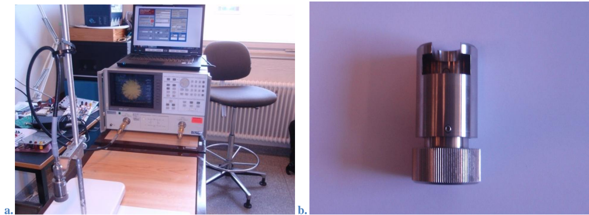
Figure 10. The experimental setup for the coaxial reflection measurements, a. The whole setup consists of the network analyzer, a computer, the coaxial probe with the short standard on it, b. The short standard.
