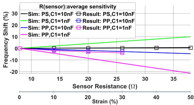
Figure 4.4: Frequency behaviour caused by variations in  $R_{sensor}$ .
