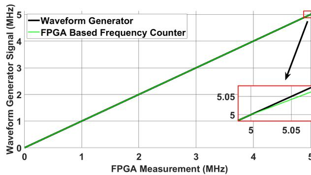
Figure 3.26: Accuracy of the FPGA implemented frequency counter.
