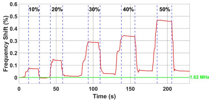
**Figure 4.1:** Systematically induced strain on  $R_{sensor}$  with the PS topology  $C_1 = 10$  nF.
