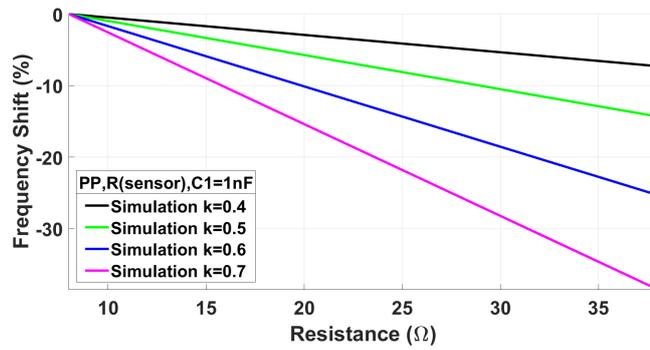
**Figure A.4:** LTspice simulations for variations in  $R_{sensor}$  with the PP topology and  $C_1 = 1$  nF. The simulated values for  $k=0.8$  and  $0.9$  showed unrealistic behaviour and were removed.
