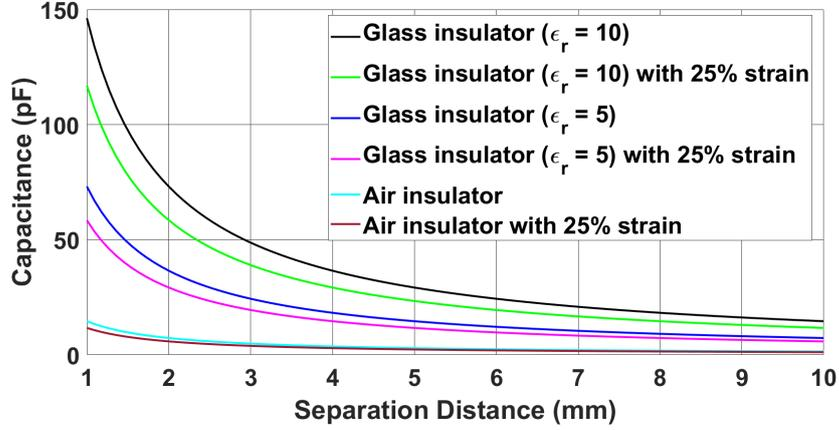
Figure 2.13: Parasitic capacitance between two square planar coils.
