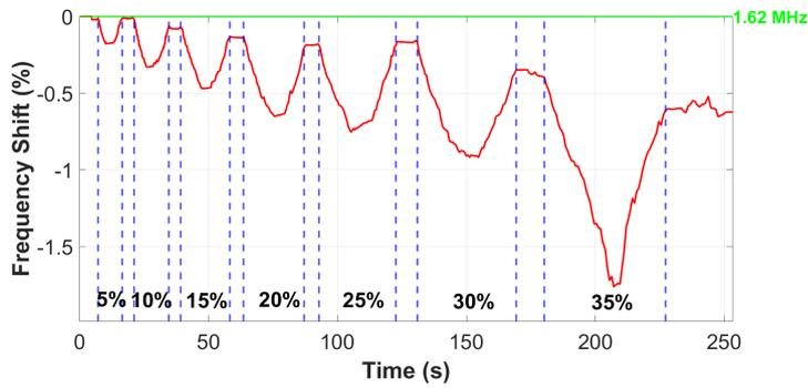
**Figure A.17:** Systematically induced strain on  $C_2$  with the PS topology and  $C_1 = 10$  nF.
