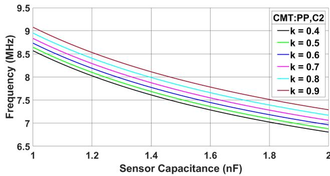
**Figure 3.17:** Frequency shift caused by variations in sensor capacitance of a PP topology circuit according to coupled mode theory.
