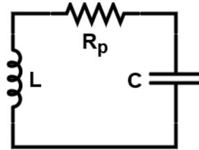
Figure 2.15: Model for visualizing  $R_p$  in a spiral inductor coil.
