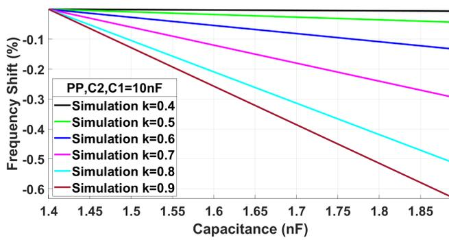
**Figure A.7:** LTspice simulations for variations in  $C_2$  with the PS topology and  $C_1 = 10$  nF.
