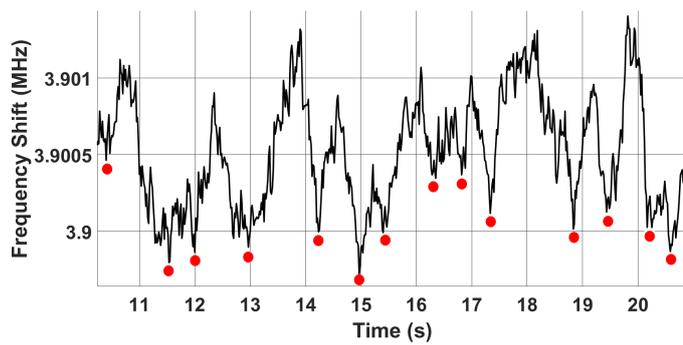
Figure 4.7: Pulse wave detection test using a parallel RLC circuit with a reader capacitor of 1 nF.
