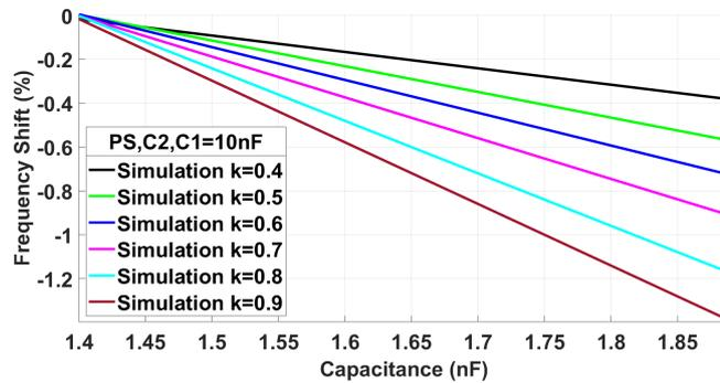
**Figure A.5:** LTspice simulations for variations in  $C_2$  with the PS topology and  $C_1 = 10$  nF.
