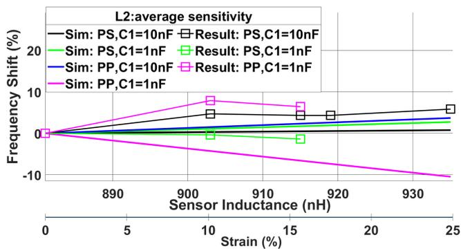
Figure 4.6: Frequency behaviour caused by variations in  $L_2$ .
