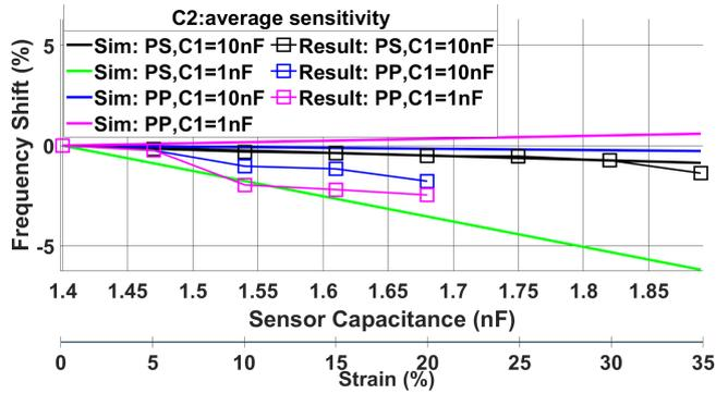
Figure 4.5: Frequency behaviour caused by variations in  $C_2$ .
