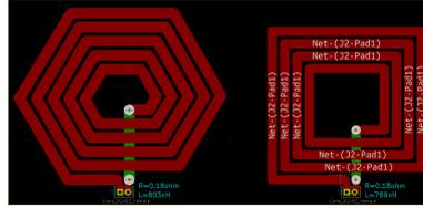
**Figure 2.10:** KiCad designs of spiral planar coil inductors.
