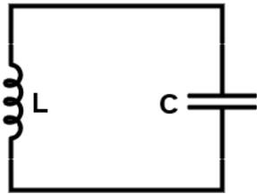
Figure 2.14: LC resonator.
