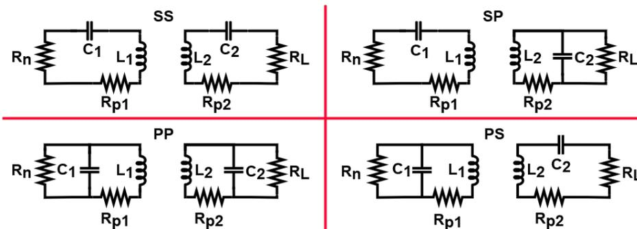
**Figure 2.1:** Circuit topologies for RLC based WPT systems.
