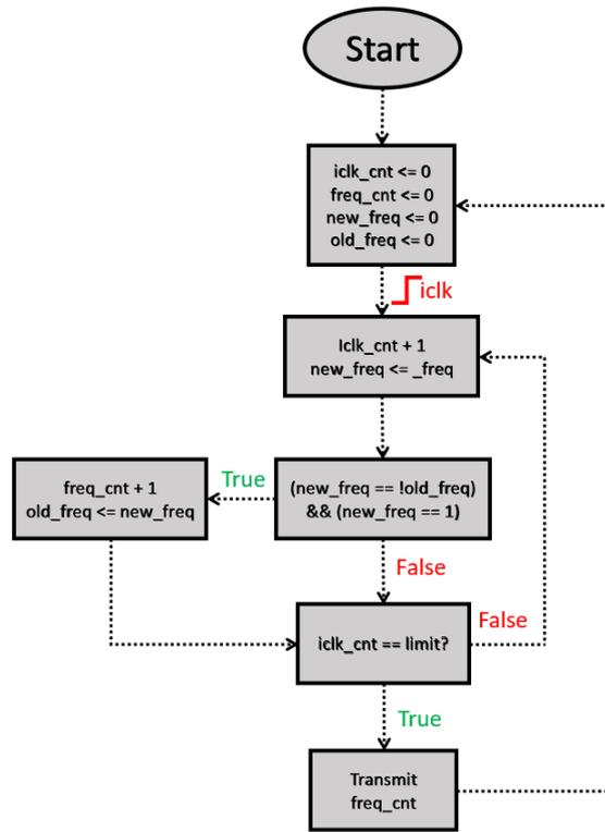
Figure 3.25: State diagram of the FPGA implemented frequency counter.
