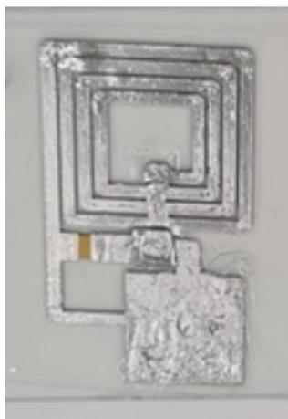
**Figure 3.28:** Stretchable parallel RLC sensor,  $R_{sensor} = 2 \Omega$ ,  $L_2 = 881 \text{ nH}$  and  $C_2 = 1.4 \text{ nF}$ .
