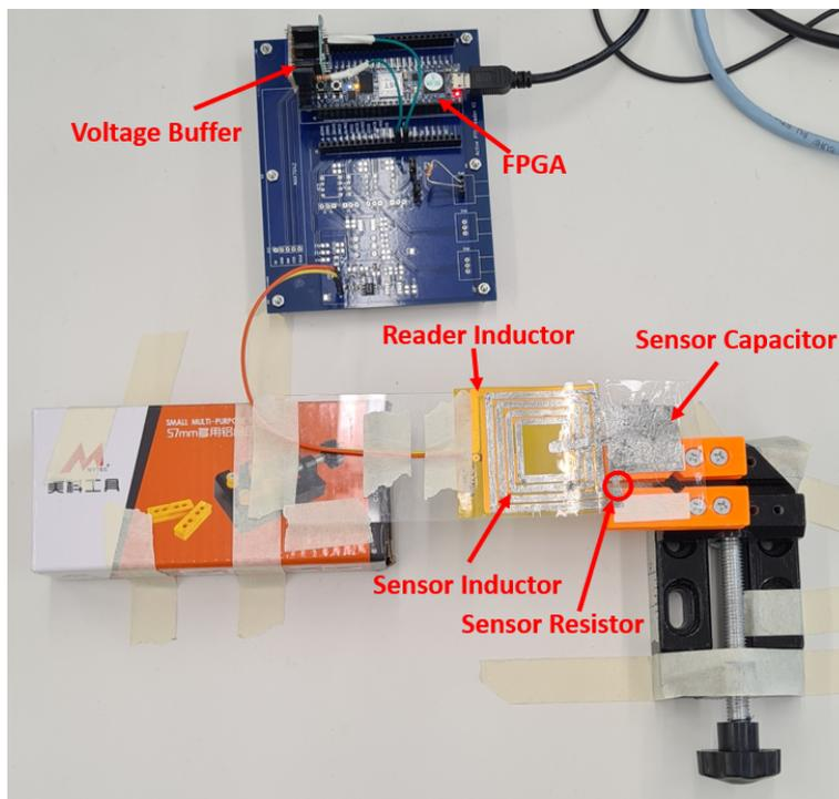
**Figure 3.27:** Measurement setup for systematic resistive strain.
