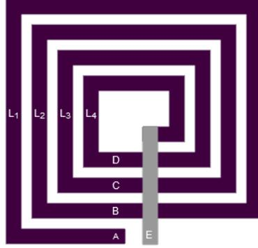
**Figure 2.8:** Model for visualizing the total inductance.
