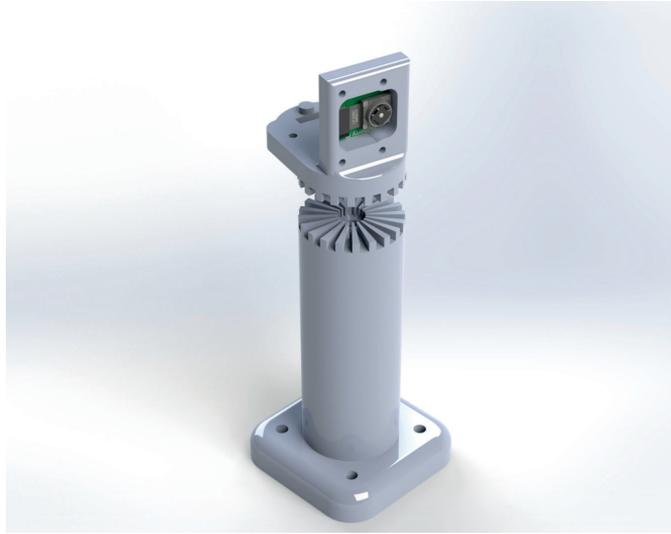
**Figure 3.12:** Camera mount consisting of two parts to be able to adjust direction in increments of  $16^\circ$ .
