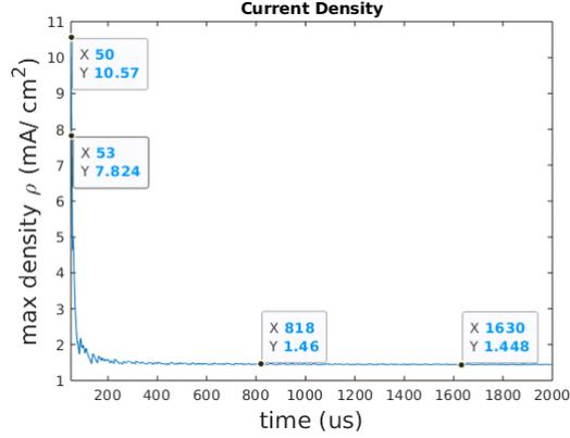
**Figure 3.4:** Max Current Density evolution during one pulse
