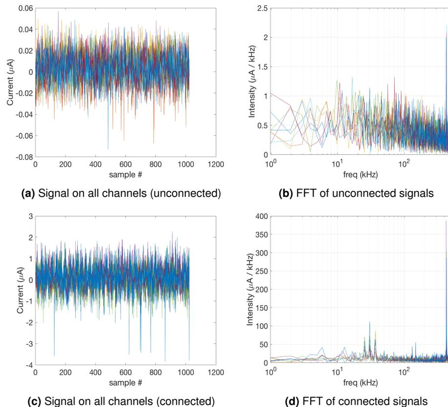
**Figure 2.13:** Current signals acquired by the FMC
