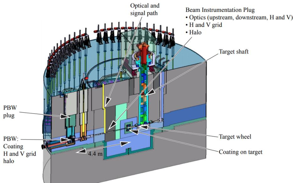
**Figure 2.6:** Location of Beam on Target instrumentation electronics [1]
