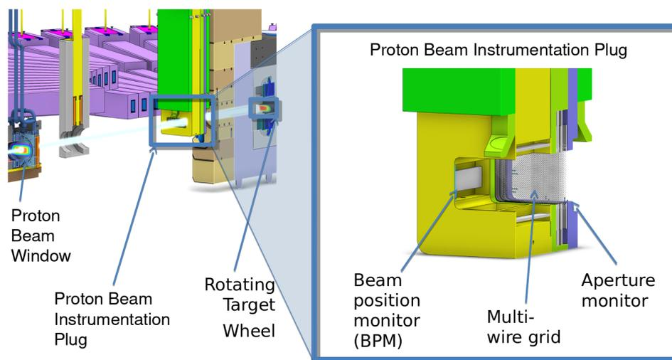
**Figure 2.7:** Beam on Target instrumentation electronics at PBIP [3]
