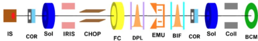
**Figure 2.5:** Schematic of Beam Instrumentation in LEBT [2].
