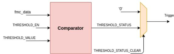
**Figure 4.2:** Hardware implementation of the APTM algorithm
