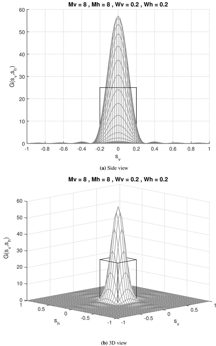
**Figure 3.17:** UPA that uses Slepian, with 8 antenna elements activated on each dimension, and  $W_v = W_h = 0.2$ , intended to cover a region 0.2 on each direction. The region is indicated by lines.
