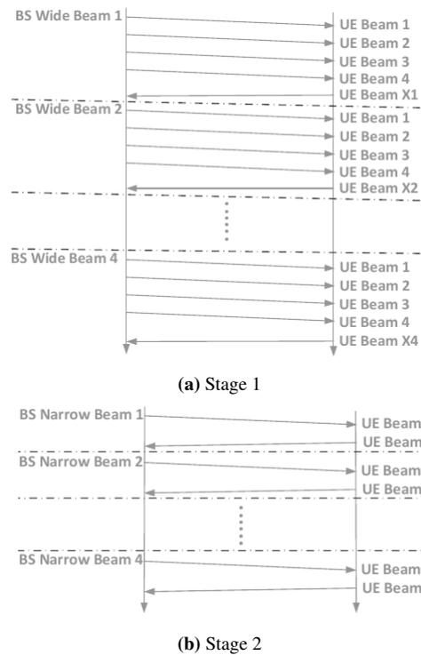
**Figure 2.7:** (a) Iterative beam sweeping procedure. 4 wide beams in the BS codebook stage 1, and 4 beams in the UE codebook. (b) 4 narrow beams used from the BS codebook stage 2 that correspond to the selected wide beam in stage 1, and 1 beam used from UE codebook (The best from stage 1). [Images source: 11].
