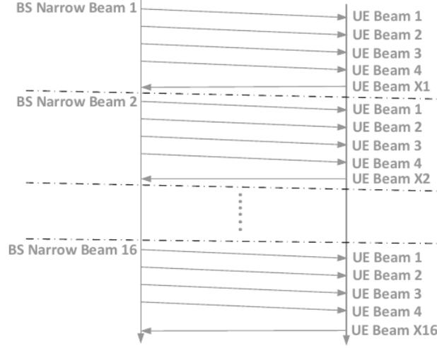
**Figure 2.6:** Exhaustive beam sweeping procedure. 16 beams in the BS codebook, and 4 beams in the UE codebook [Image source: 11].
