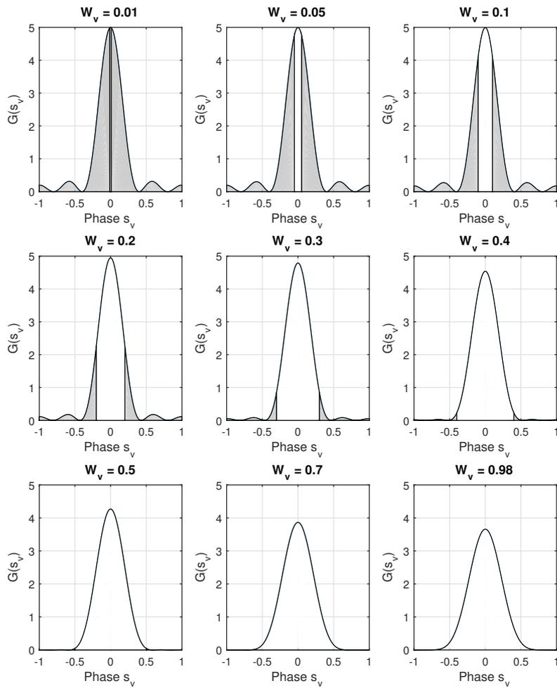
**Figure 3.4:** The radiation pattern of the Slepian beam of 5 antenna elements, scanned across selected values of  $W_v$ , starting from DFT and ending with binomial. The patterns are drawn in the phase domain. The width of the targeted area [white area] is  $2W_v$ .
