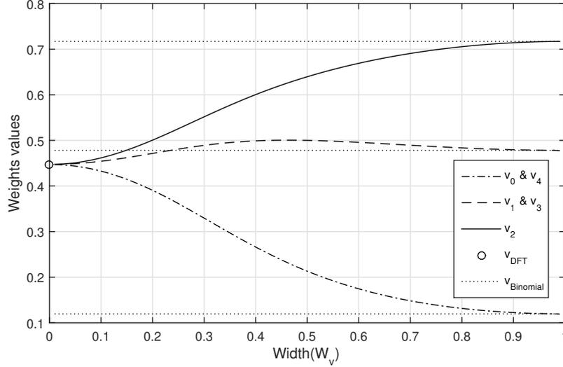
**Figure 3.3:** The weights of a 5 antenna elements Slepian beam scan from  $W_v = 0$  where they converge to DFT, to  $W_v = 1$  where they converge to binomial.
