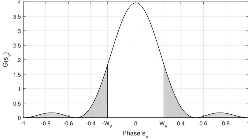
**Figure 3.2:** Arbitrary radiation pattern shows area under the radiation pattern for the target region [white], and outside [grey]. The white area needs to be maximized, and the grey area needs to be minimized.
