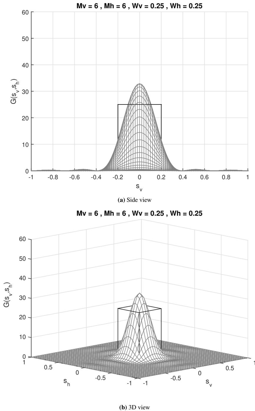
**Figure 3.16:** UPA that uses Slepian, with 6 antenna elements activated on each dimension, and  $W_v = W_h = 0.25$ , intended to cover a region 0.2 on each direction. The region is indicated by lines.
