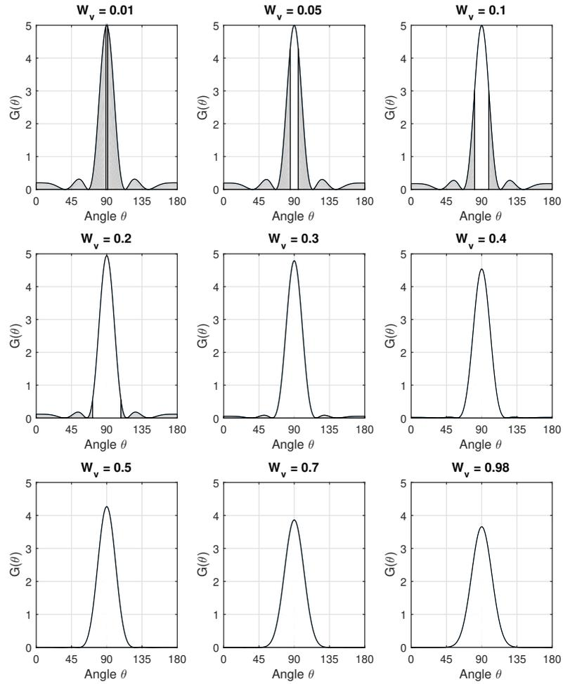
**Figure 3.5:** The radiation pattern of the Slepian beam of 5 antenna elements, scanned across selected values of  $W_v$ , starting from DFT and ending with binomial. The patterns are drawn in the angular domain. The width of the targeted area [white area] is  $2 \cos^{-1}(W_v)$ .
