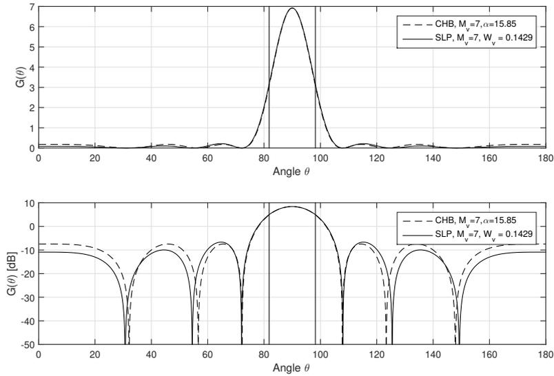
**Figure 3.11:** Radiation patterns of a ULA that uses Slepian/Chebyshev beams (7 antenna elements).
