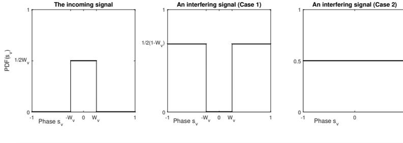
**Figure 3.6:** Phase distribution of the incoming signal [Left] and an interfering signal. There are two cases of interference distribution [Mid, Right].
