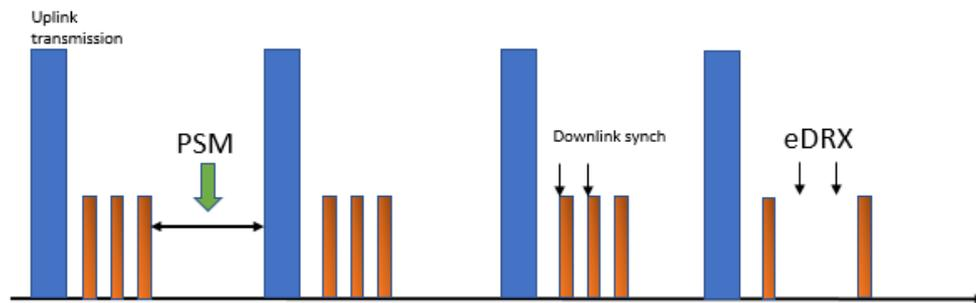
**Figure 2.12.** Power Saving methods in NB-IoT
