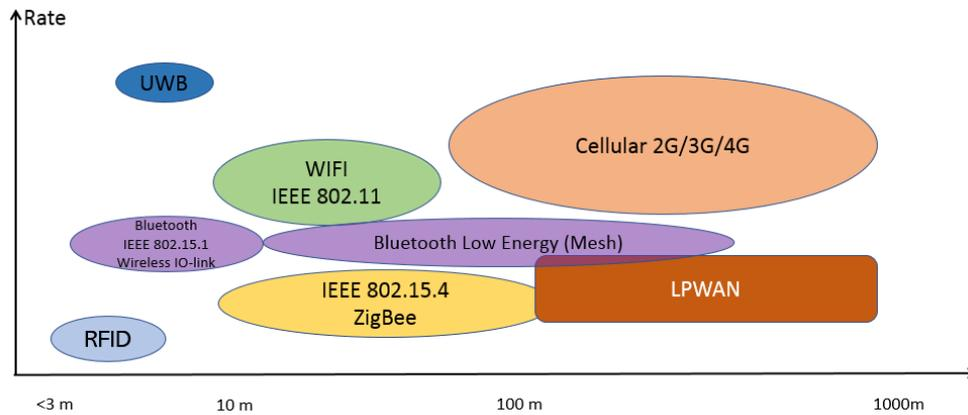
**Figure 1.1.** Coverage and Transmission Rate (bps) Comparison among Wireless Technologies
