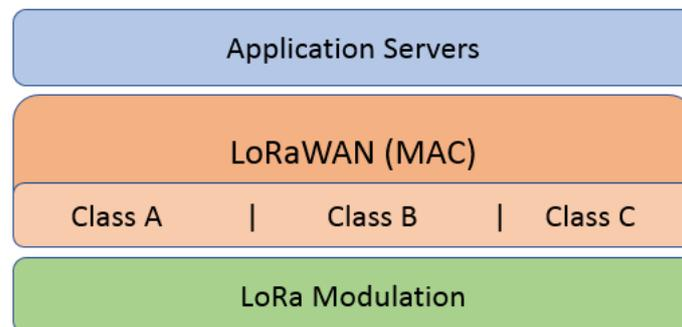
**Figure 2.7.** LoRa and LoRaWAN Layers
