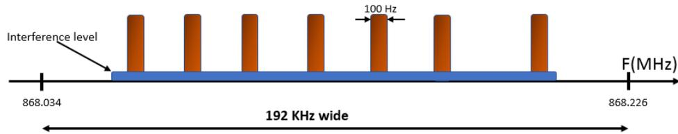
**Figure 2.1.** UNB Modulation Technique & Interference Resilience
