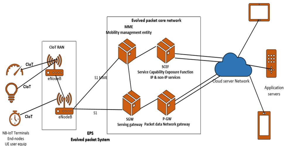
**Figure 2.14.** NB-IoT Network architecture
