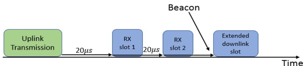
**Figure 2.9.** Class-B End-Devices
