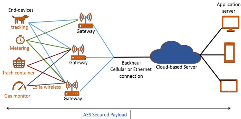
**Figure 2.11.** LoRaWAN Network Architecture
