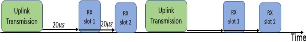
**Figure 2.8.** Class-A End-Devices
