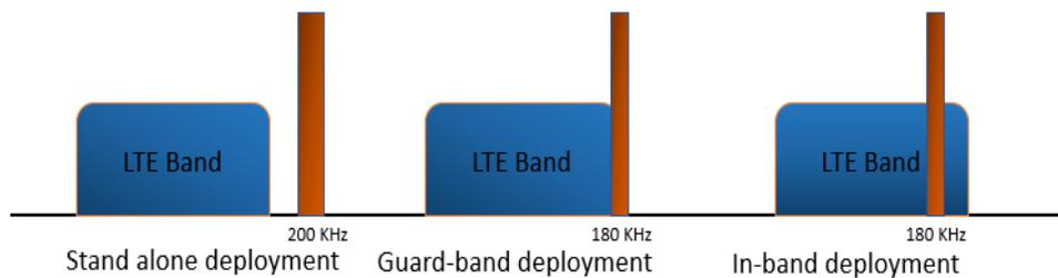
**Figure 2.13.** Deployment Modes in NB-IoT
