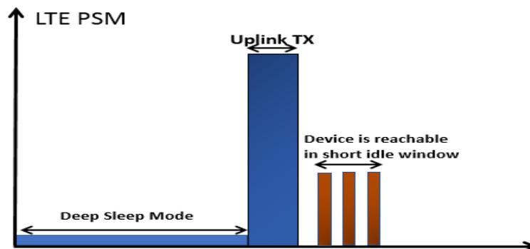
**Figure 2.16.** LTE Power Sleeping Mode (PSM)
