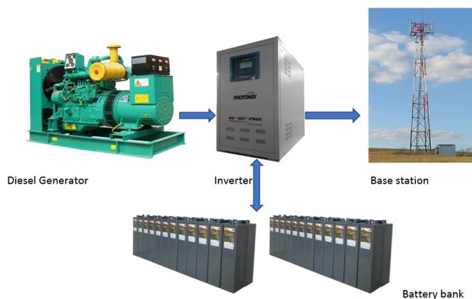
**Figure 5.12:** Fully diesel powered site set up
