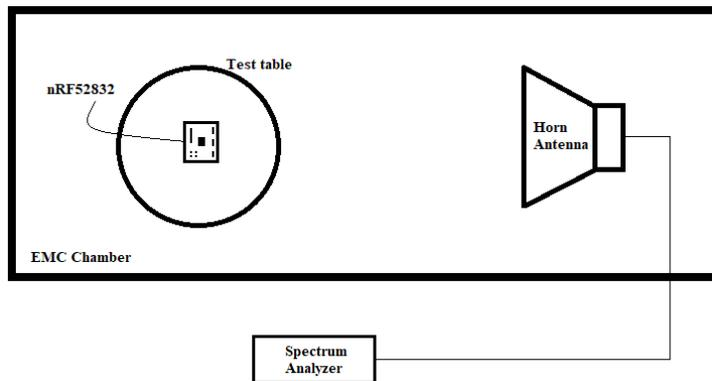
Fig. 2. A basic sketch of the test environment. This is the setup for the reference measurement. When the protection box, the container and pot was used in the test they were added at the table and adjusted in a way so that the position of the chip was not changed.
