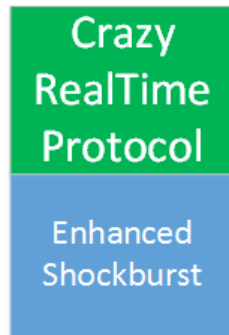
Figure 4. The network stack of both the Crazyradio and Crazyflie. Enhanced Shockburst is the physical layer and Crazy Real Time Protocol is a layer above it.
