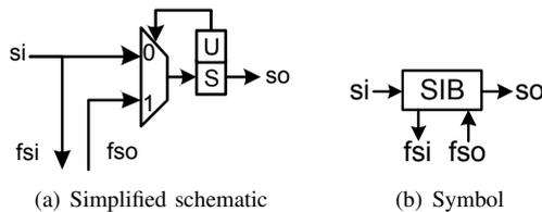
Fig. 2. Segment Insertion Bit (SIB)
