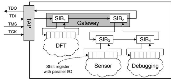
Fig. 4. A 1687 network with three instruments inside a chip
