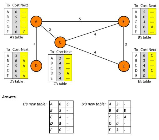
1.2. **[6 points]** Use once again the initial network topology shown in the diagram above. (Ignore all routing tables and the extra link added in the previous question.) Assume that the whole topology is known to all the nodes after the flooding of the individual "link state" knowledge. Perform the shortest path tree algorithm used in OSPF, draw the tree step-by-step and derive the routing table for node E.
