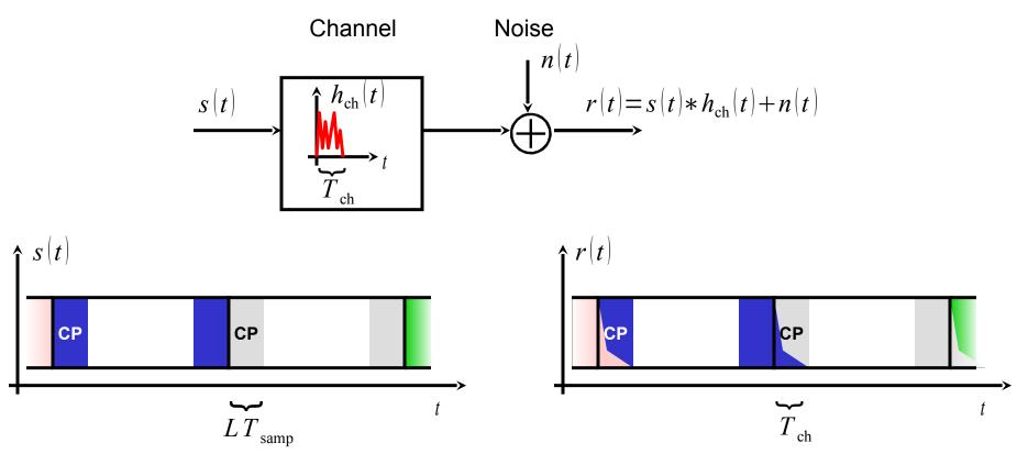
As long as the CP is longer than the delay spread of the channel,  $LT_{samp} > T_{ch}$ , it will absorb the ISI.
