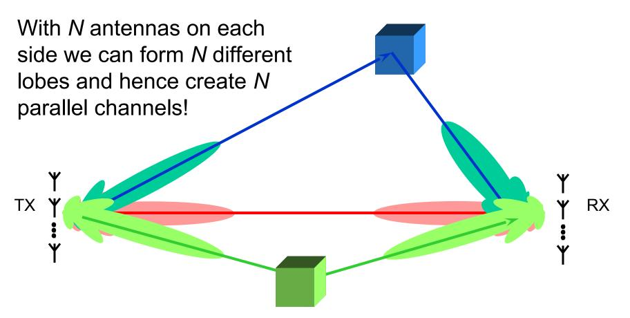
Note that the three channels are separated spatially and can therefore use the same bandwidth! We have "trippled" the channel capacity.
