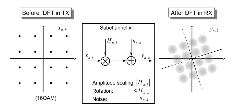
• Simple equalization of each subchannel: Back-rotate and scale
