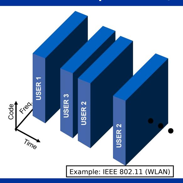
Users are separated in time but not in an organized way. The terminal listens to the channel, and transmits a packet if it's free.
