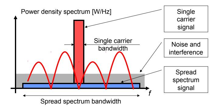
Using a bandwidth expansion M, the spread spectrum signal has M times greater bandwidth and M times lower power spectral density. (M is also called the processing gain)
