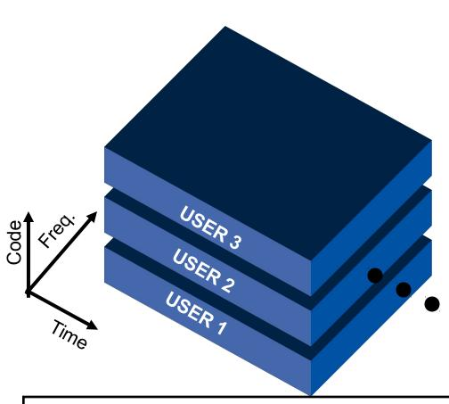
Users are separated by spreading codes.
