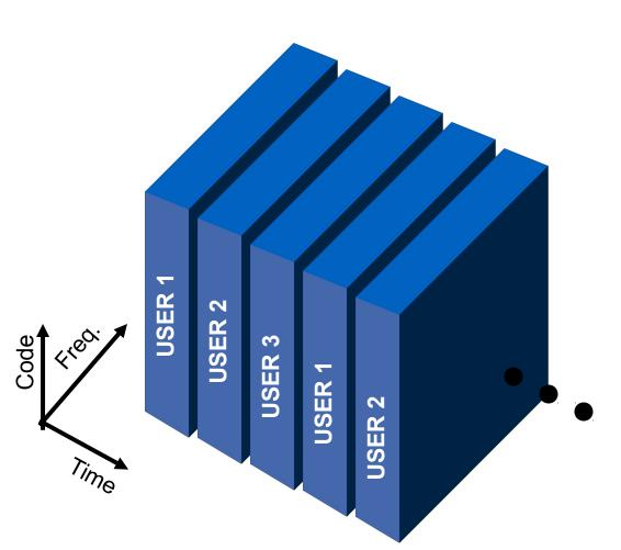
TDMA is usually combined with FDMA, where each frequency channel is subdivided in time to provide more channels.
