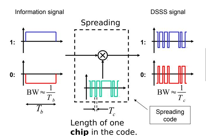
Users/channels are separated by using different spreading codes.
