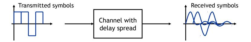
ISI will degrade performance of our receiver, unless mitigated by some mechanism. This mechanism is called an **equalizer**.
