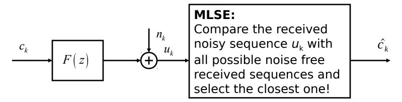
For sequences of length N bits, this requires comparison with  $2^N$  different noise free sequences.
