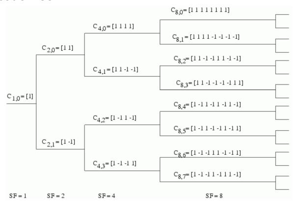
We can create several orthogonal channels by picking spreading codes from different branches of the tree.
