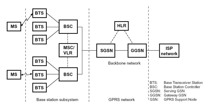
SGSN Serving GPRS Support Node GGSN Gateway GPRS Support Node ISP Internet Service Provider
